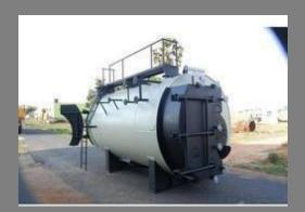
Huskpac Series, the next generation rice husk fired boilers from Steamgen & C.,, are designed to provide low cost heating with fuel efficiency as high as 74 %. Bubbling bed combustion, gives higher residence time to facilitate complete combustion, thus improving efficiency.
